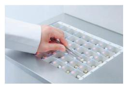
The LED light will indicate the position to set the medications. It allows users to reduce human error
